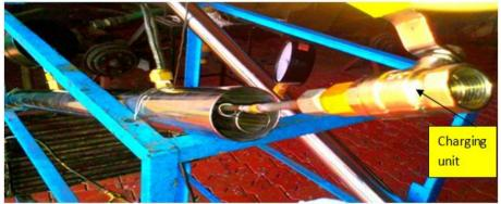
Fig. 2 Adsorber (Bed A) with charging unit
